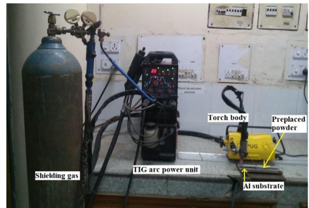
Fig. 2 Experimental set-up of TIG arc surfacing
