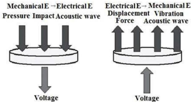
Fig 9. Piezoelectric and reverse Piezoelectric effect
