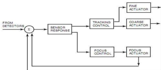
Fig 4. Block diagram of the servocontrol system for an optical disk drive.
