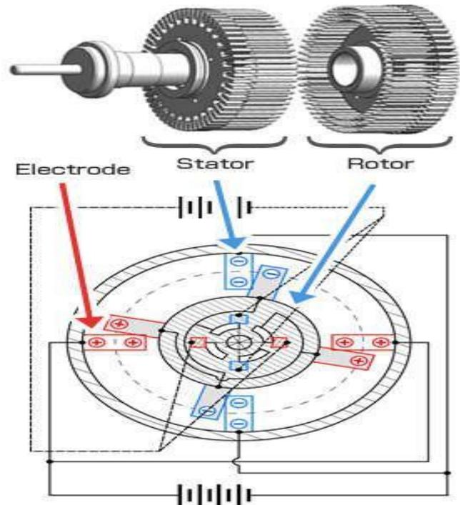
Fig 5. Arrangement of Electrostatic Motor (Shinsei Corporation Japan)
