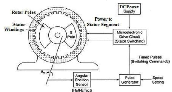
Fig 3. System of Brushless DC Generator
