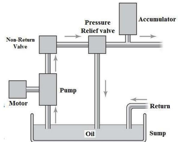
Fig 8. Hydraulic Actuation system
