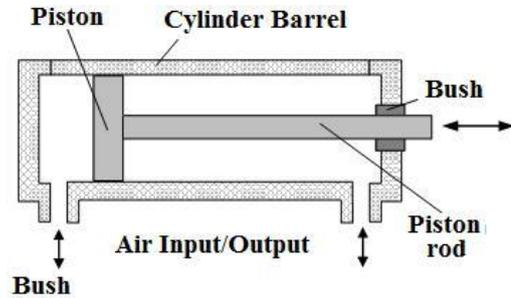
Fig 7. Pneumatic Actuation system (cylinder)
