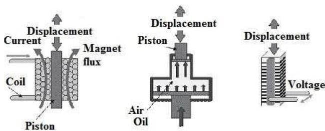
Fig 2. Mechanisms of various Actuating systems
