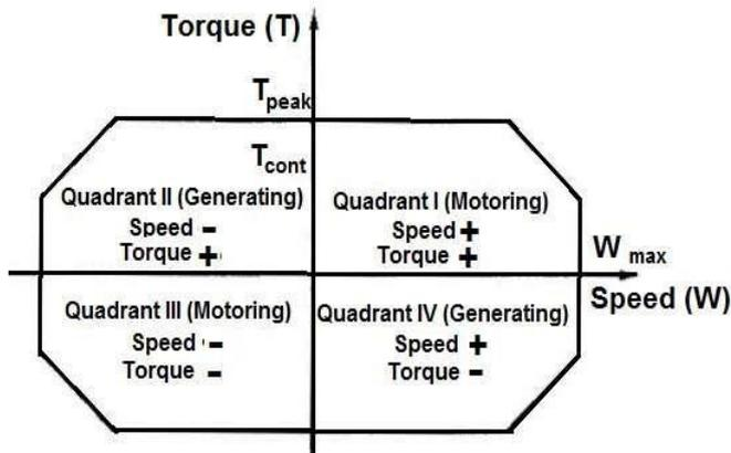
Fig 6. Torque Vs Speed characteristics of an Electric motor.
