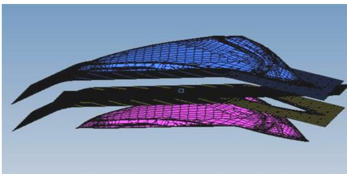
Fig. 5. Assembly of the (1) Die at the top, (2) Blank, (3) Binder and the (4) Punch at the bottom
