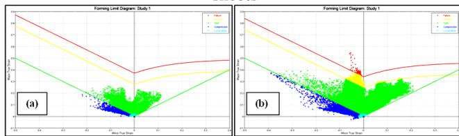
Fig. 8. Forming limit plots for (a) IF and (b) DDQ steel sheets
