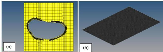
Fig. 4. (a) Binder and (b) Blank after meshing using HYPERMESH
