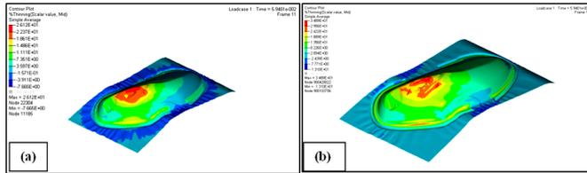
Fig. 7. Thinning contour plots for (a) IF and (b) DDQ steel sheets
