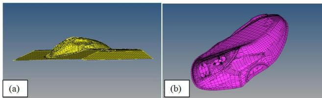
Fig. 3. (a) Die and (b) Punch after meshing
