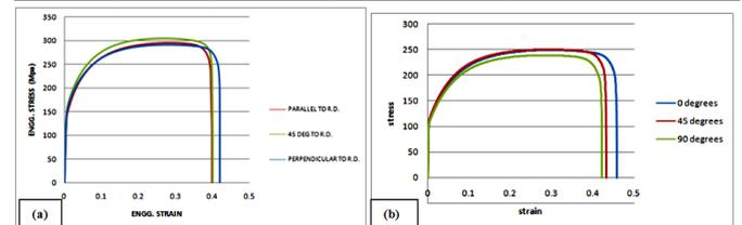
Fig. 6. Engineering Stress and strain plots for (a) DDQ and (b) IF steel sheets
