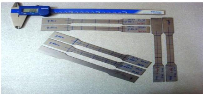
Fig. 1. Tensile test specimens in 0°, 45° and 90° w.r.t. the rolling direction
