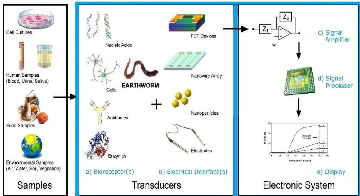
**Figure:1-Elements of a Biosensor**
