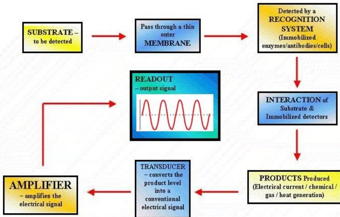
Figure:2-Process Flow diagram of a biosensor
