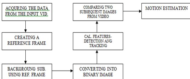
Fig 1: The key stages in the vehicle identification
