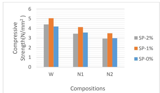
Figure 2 – Compressive strength for mortar 1:4 for 14days
