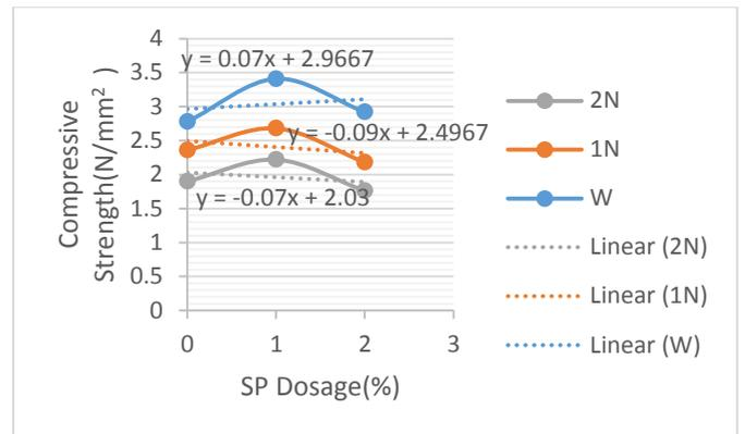
Figure 8– Compressive strength for mortar 1:6 for 14days
