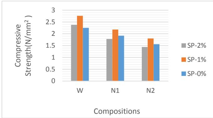
Figure 3 – Compressive strength for mortar 1:6 for 7days
