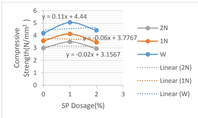
Figure 6– Compressive strength for mortar 1:4 for 14days
