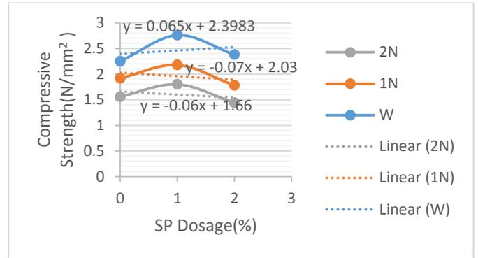
Figure 7 – Compressive strength for mortar 1:6 for 7days
