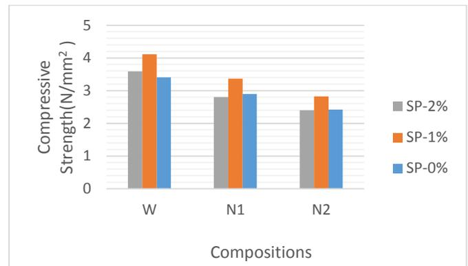
Figure 1 – Compressive strength for mortar 1:4 for 7 days
