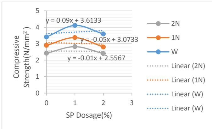
Figure 5 – Compressive strength for mortar 1:4 for 7 days
