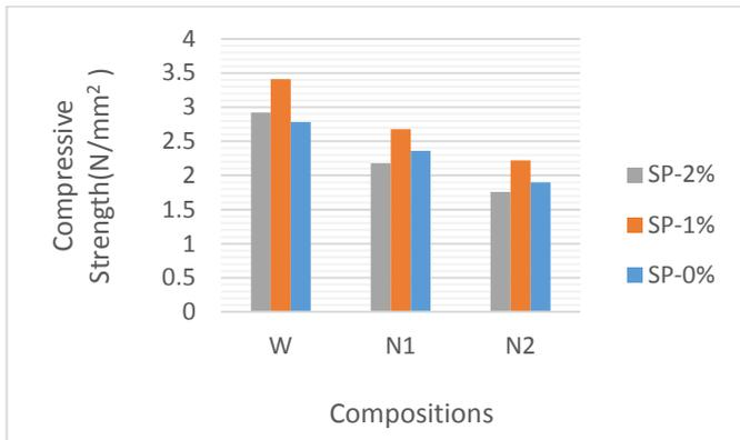
Figure 4 – Compressive strength for mortar 1:6 for 14days
