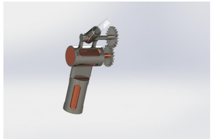
Fig. 3 Slave Manipulator performing Ultrasound (View Of Wrist)
