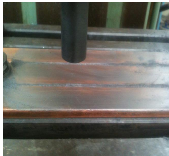
Fig. 3 CNT filled in the grooves of copper plate
