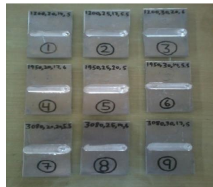
Figure 4. Plate after friction stir welding
