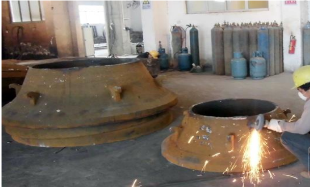
Fig. 7 Trimming and grinding[15]
