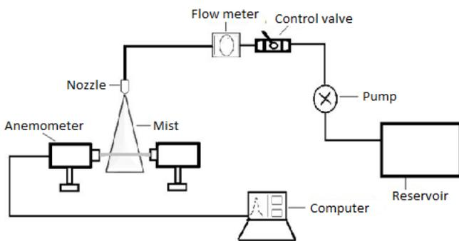
**Figure 2.** Experimental setup
