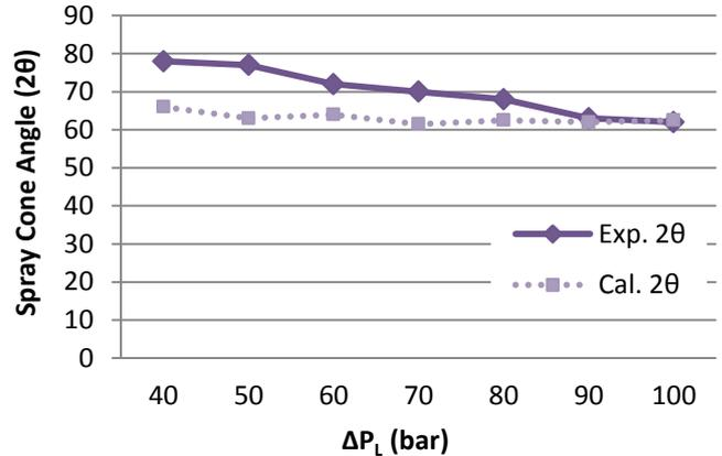
Figure 6. Variation of spray cone angle ( $2\theta$ ) with varying  $\Delta P_L$
