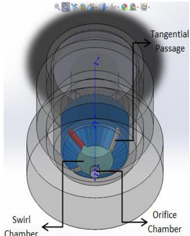
**Figure 4.** Solid Works 3D model of the atomizer
