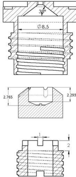
**Figure 3.** Cross section of the atomizer
