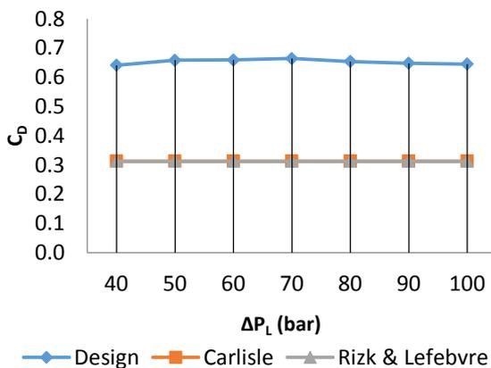
Figure 5 b. Experimental discharge coefficient Vs pressure difference
