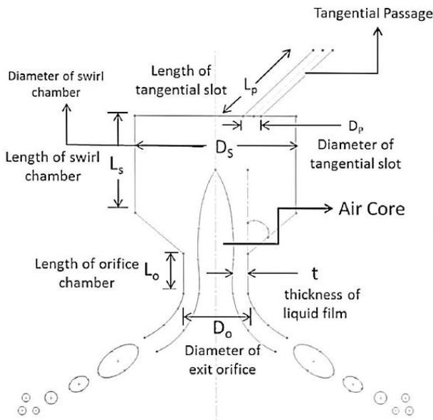
**Figure 1.** Schematic of Pressure swirl atomizer
