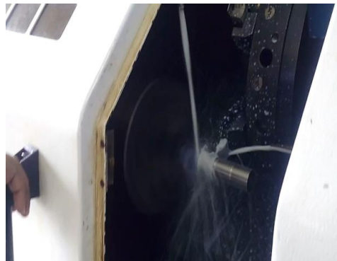
Fig2. Experimental setup for CNC Wet turning.
