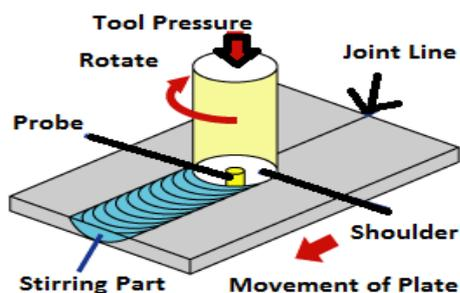
Figure 1: Friction Stir Welding Process
