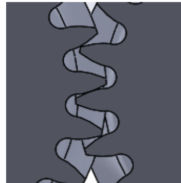
Figure 2. Helical gear model for \varphi_d = 20^\circ, \varphi_c = 20^\circ, \beta = 15^\circ
