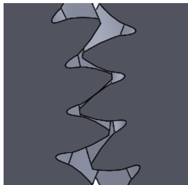
Figure 6. Helical gear model for \phi_d = 40^\circ , \phi_c = 20^\circ , \beta=15^\circ
