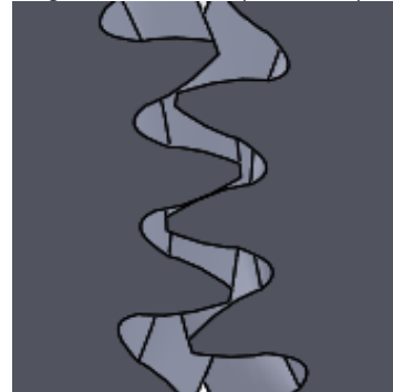
Figure 3. Helical gear model for \varphi_d = 25^\circ, \varphi_c = 20^\circ, \beta = 15^\circ
