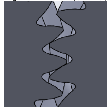
Figure 4. Helical gear model for \varphi_d = 30^\circ, \varphi_c = 20^\circ, \beta = 15^\circ (Symmetric gear)
