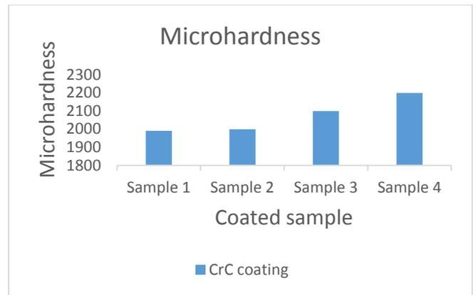
Fig. 2 Shows variation of microhardness of CrC coating
