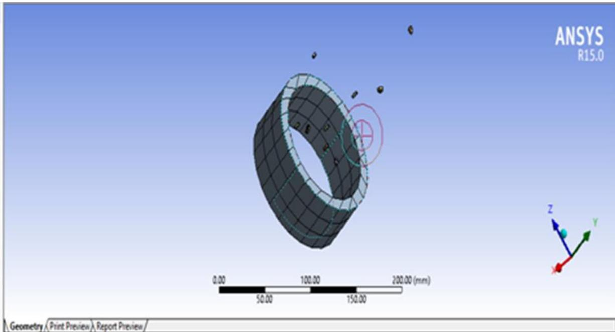
Figure 4 Meshing of Workpiece and Abrasives
