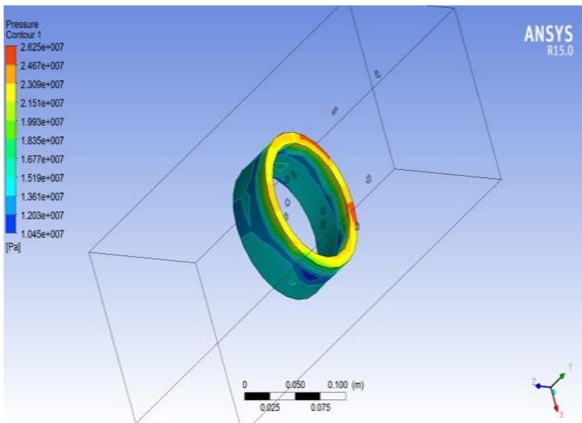
Figure 6 Pressure Variation on Workpiece'
